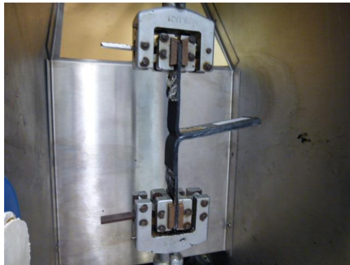
Figure 2: Picture of peel test made by tensile testing machine.
