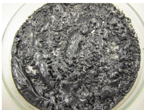
Figure 2 – Melted Organosolv lignin after exposure @ 150 °C
