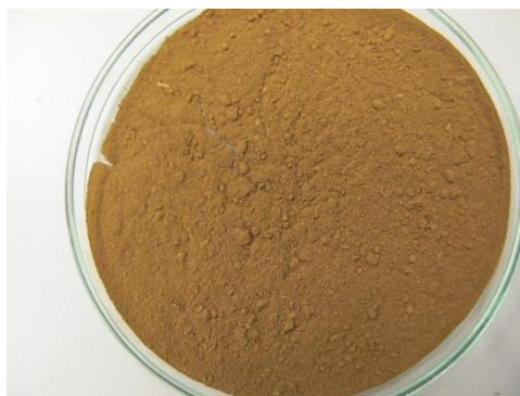
Figure 1 – Example of a powder, filler-like type of lignin
