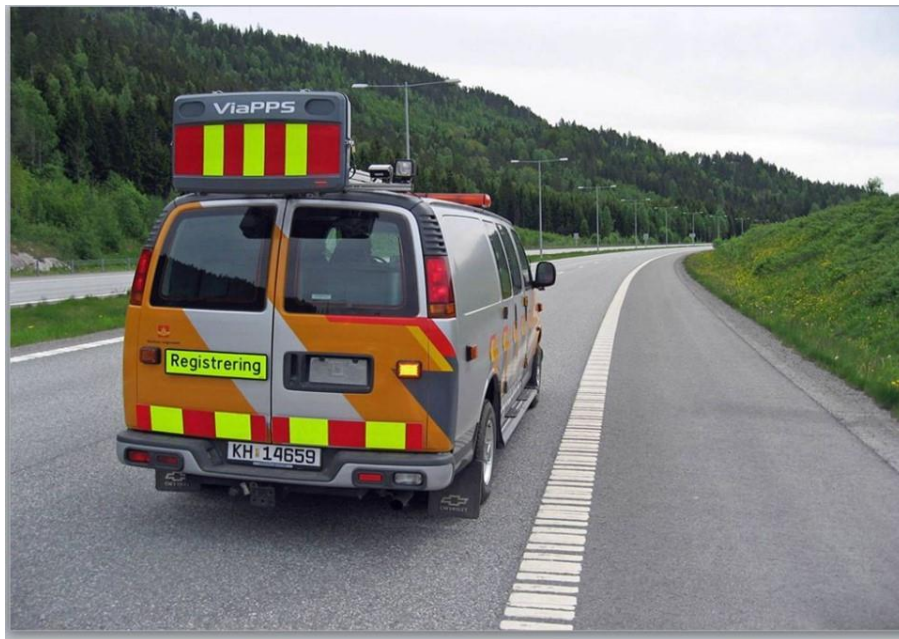
Figure 1: NPRA's mobile road profile scanner for measurement of rutting
